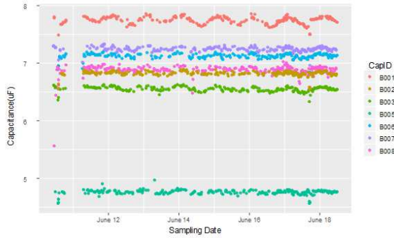
Fig. 6. C_{CN} of each capacitor of B phase
